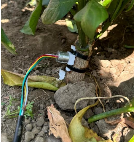
Pepper installation with 3D printed jig that holds the sleeve in place.
