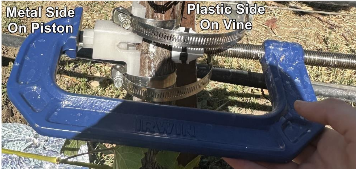
Press into place with C-clamp
