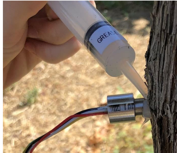
Add sealant (not grease, photo outdated)
