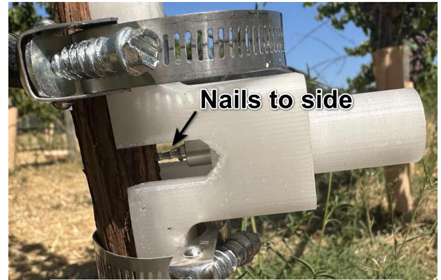
Place piston inside guide and align
