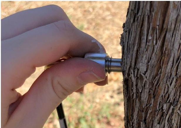
Insert probe and follow with cap.
