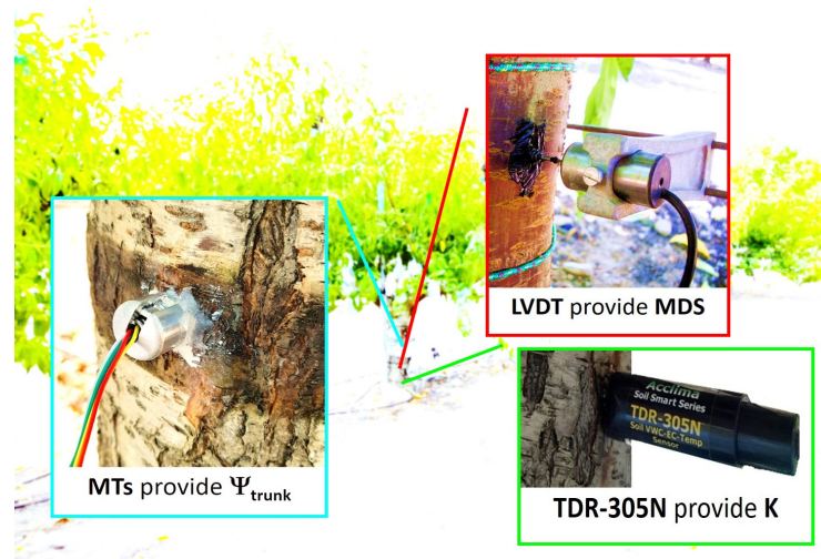
Figure 1. Details of plant biosensors (MTs, TDR-305N, and LVDT) installed on a nectarine tree trunk.
