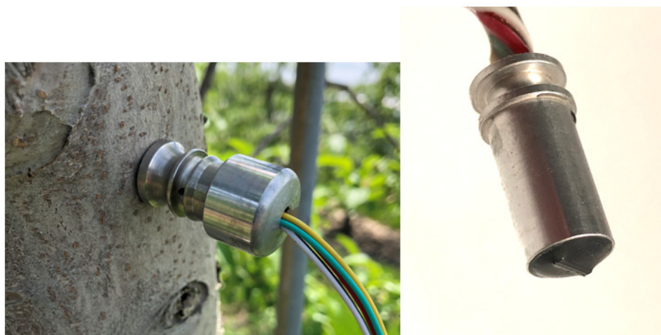
Figure 1. The sensor probe installed with support sleeve in an apple tree prior to sealing and insulation. The probe also houses the associate electronics.
