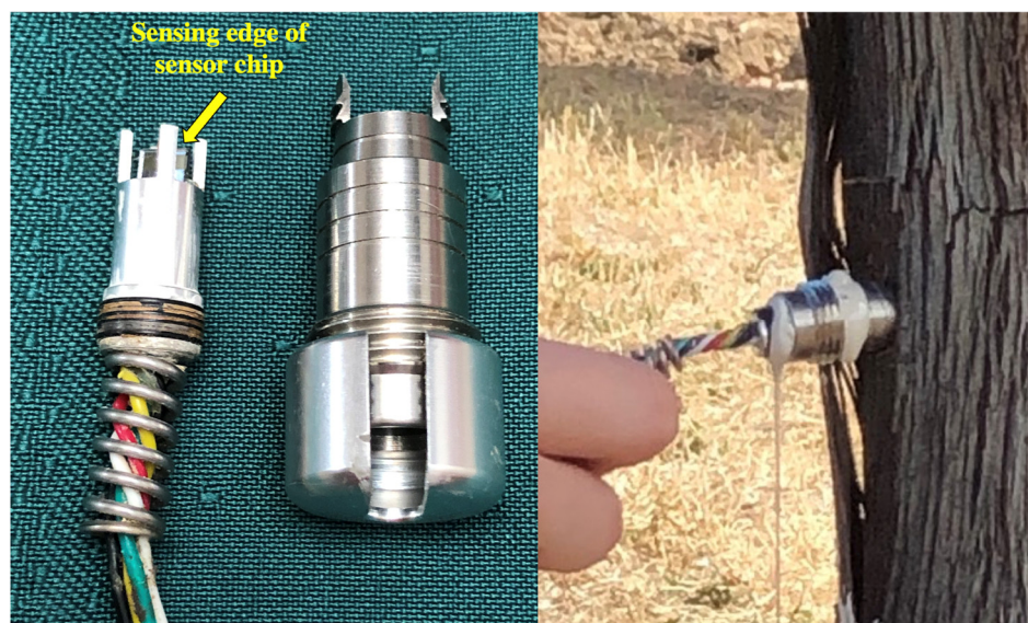
Figure 2. Photographs of the FloraPulse microtensiometer and installation. The sensing edge of the chip is held in a probe and held in contact with the xylem by the outer steel sleeve. After driving the sleeve into the stem, the sleeve is a drill guide, and a liquid clay paste is injected before the sensor probe is inserted. The nut of the sleeve then holds the spring-loaded probe in position.
