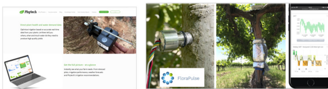
Figure 3. Left) Phytech website page showing the dendrometer attached to the stem and the app provided to the users (Phytech.com); Right) A FloraPulse sensor is installed in a tree stem and information is presented in an app (FloraPulse.com). Note that for both companies, the water status is colour-coded based on an understanding of the impact of the water status on tree physiology and performance.
