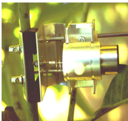
Figure 1. (Left) A microdendrometer using LVDT sensor (Linear variable displacement transducers, PEPISTA, France) installed on a twig of a mango tree; (Right) Diurnal changes in the diameter of a branch (red, pointed line) and fruit (black, unbroken line) on a 3-year-old mango ('Kensington Pride') tree grown in a 200L plastic drum. Irrigation was turned off from September 23, 1996 onwards, in Darwin, Australia (Lu, 2006).
